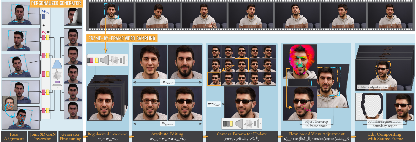
Figure 2. VIVE3D Pipeline. To create an edited video, we first need to create a personalized generator by jointly inverting selected faces and fine-tuning a pre-trained generator. We then invert the cropped face regions from a source video (which could be the same or a different video) into our personalized generator and recover the latent codes and camera poses for each target frame. We are able to perform semantic editing on the inverted stack of latent codes using previously discovered latent space directions and we can freely change the camera path around the face region. In order to composite the face with the source frame in a consistent fashion, we use optical flow to correct the position of the inset within the frame, which allows us to composite the result in a seamless and temporally consistent fashion.
