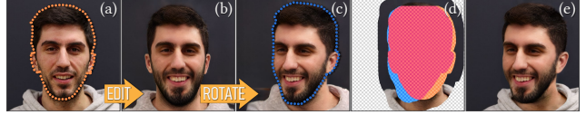
Figure 5. Border Composition. We calculate the composition border based on face segmentations of the target image (a) and the edited inset (c). We unite the masks and dilate the resulting joint mask to obtain a boundary around the face regions (d) that should be optimized, which allows us to create the final composition (e).
