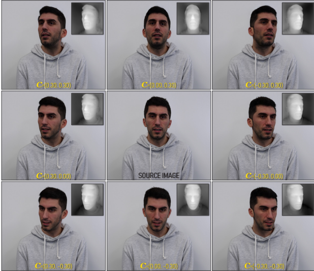
Figure 8. Changing camera poses. Our method can freely alter the camera pose and composite the result back with the source frame by fixing the divergence between the source and target pose using our optical flow correction strategy. The generated results look natural despite the static body pose.
